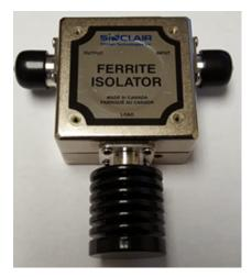
Figure 4: The circulator becomes an isolator when a matched 50-ohm load is added
