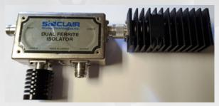
Figure 6b: Dual isolator type "B"
