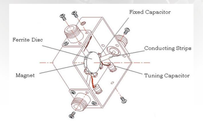
Figure 2: The internal materials of a typical ferrite circulator
