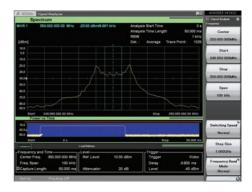
Figure 68: 2-FSK signal spectrum (Signal analyzer)
