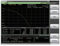
Figure 17: Example of CCDF trace (CCDF of terrestrial digital TV signal)
