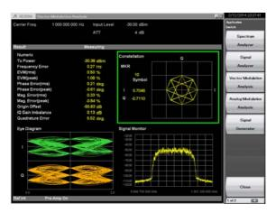
Figure 108: 1074-DQPSK modulation with an AWGN overlay and ~20 % EVM (peak)
