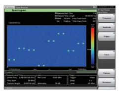
Figure 18: Example of Spectrogram trace (Frequency hopping of Bluetooth signal)
