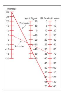
S = drive level of the input tones (signals) in dBm.
