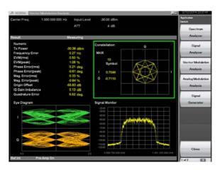
Figure 107:  $\varpi/4$ -DQPSK modulation with perfect interference free modulation and  $\sim 0\%$
