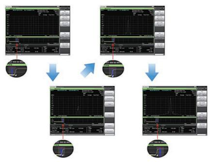
Figure 7: Sequential display of wireless signal spectrum display captured in memory
