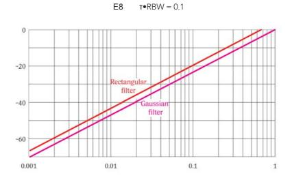
Figure 91: Amplitude loss as a function of time/bandwidth product T•B
