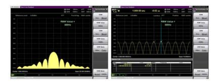
Figure 86: Left - Entire pulse within a 30 MHz Span and 300 Hz RBW resulting in a SI-Function shape
