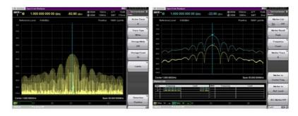
Figure 87: Pulse Spectrum for RBW of 10 kHz (left), 20 dB spectrum growth for 10 fold RBW (right)
