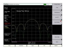
Figure 101: Test signal acc. to page 6 in Burst Detect mode
