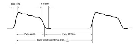
Figure 80: Pulse signal name conventions
