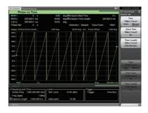
Figure 16: Example of Phase vs. Time trace (Phase characteristics of 1.9 GHz band unmodulated signal)
