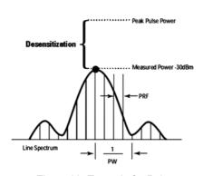
Figure 89: Example for Pulse
