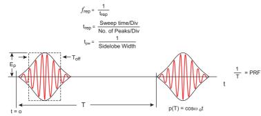
$T_{eff} = \text{Width of Rectangular Pulse of same height and area as pulse applied to analyzer} = \int_{o} \frac{p(t) \, dt}{E_{p}}$
