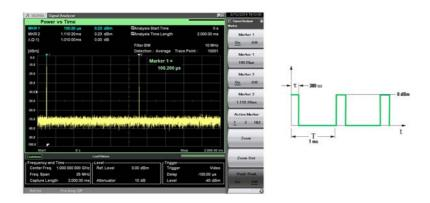
Figure 84: Measurement of 1 kHz Pulse Repetition Frequency in Power versus Time operation mode
