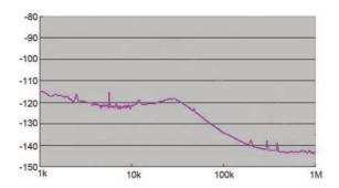
Figure 8: MS2830A Option - 066 SSB phase noise characteristics
