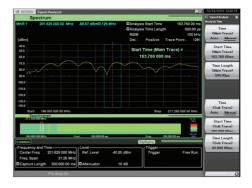
Figure 75: Instantaneous spectrum at power-on
