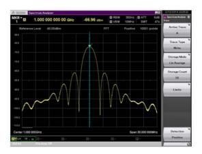
Figure 92: Line Spectrum situation - Center frequency amplitude level -66.96 dBm
