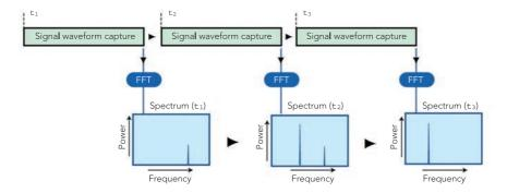
Figure 9: Continuous analysis at short cycle
