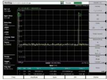
Figure 98: Narrow signal showing low duty cycle
