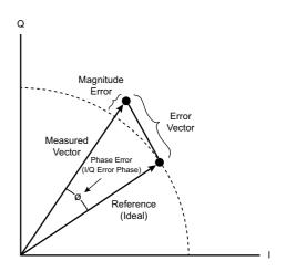
When combined with measurements of other parameters, EVM encapsulates the effects of many different signal distortions. It can therefore help pinpoint such transmission impairments as:
