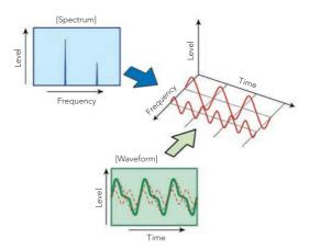
Figure 19: Signal observation direction
