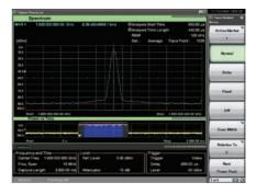
Figure 20: Example of split screen display (Main trace: Spectrum, Sub-trace: Power vs. Timel)
