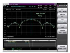
VBW = 10 MHz  $\rightarrow$  P = -66,14 dBm VBW = 10 Hz  $\rightarrow$  P = -62,74 dBm Delta:  $\rightarrow$   $\Delta$  = 3,4 dB
