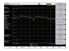
Figure 100: WiFi signal measured with Burst Detect
