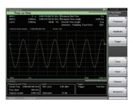
Figure 15: Example of Frequency vs. Time trace (Frequency deviation of FM waveform)
