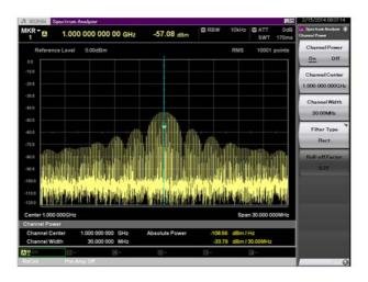
Figure 95: Average Power measurement using Channel Power feature
