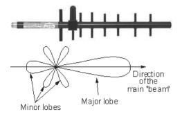
Figure 21. A Yagi antenna and its pattern.
