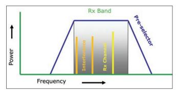
Figure 2. Interfering signals may be off-channel but inband.
