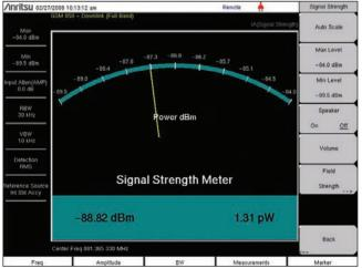
Figure 29. A Signal Strength Meter.
