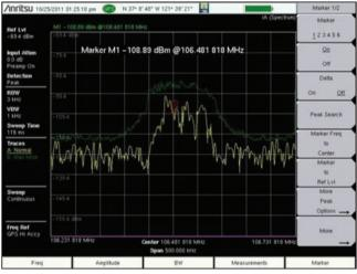
Figure 26. Signal centered on screen with Max-Hold enabled.
