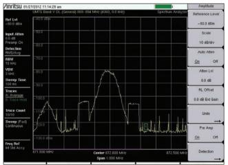
Figure 31. A fast sweep speed with good resolution.
