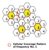
Cellular providers have a wider variety of issues. Often, they use a tiling pattern for the cells, assigning frequency or codes in this pattern, which helps control cell overlaps. Factors that can cause excessive overlap, as shown between two cells near the top of the illustration include:
