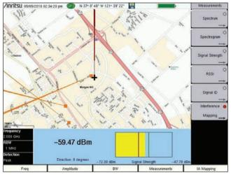
Figure 27. Plotting directions to an interference source on a map.
