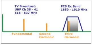
Figure 10. Harmonics can reach receive bands.
