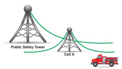
Figure 13. Near-Far problems with cellular and point-to-multi-point transmissions.
