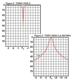
Figure 33. Notch filters or bandpass filters can cure interference problems.
