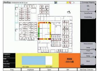
Figure 28. Plotting signal strength to find an interference source.
