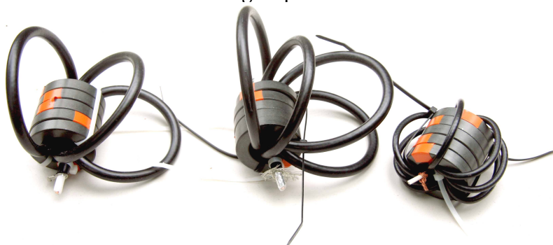
Fig 37 – Coaxial Chokes Wound to Minimize L and C
