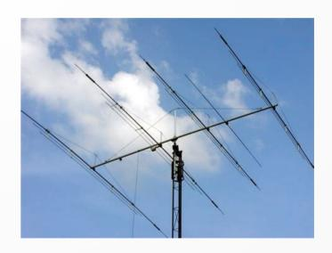
HF MULTI-BAND BEAM HORIZONTAL POLARIZATION
