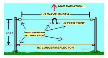
Figure 19: NVIS Configuration for Special Cases of Low Earth Conductivity
