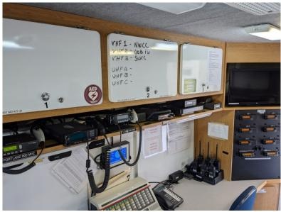
Among the communication gear in the York EMA emergency communications van are banks of VHF, UHF, and HF radios that monitor police, fire, hospital, and school radio systems. All are tied into two redundant consoles allowing up to four dispatchers to work at once if necessary.
