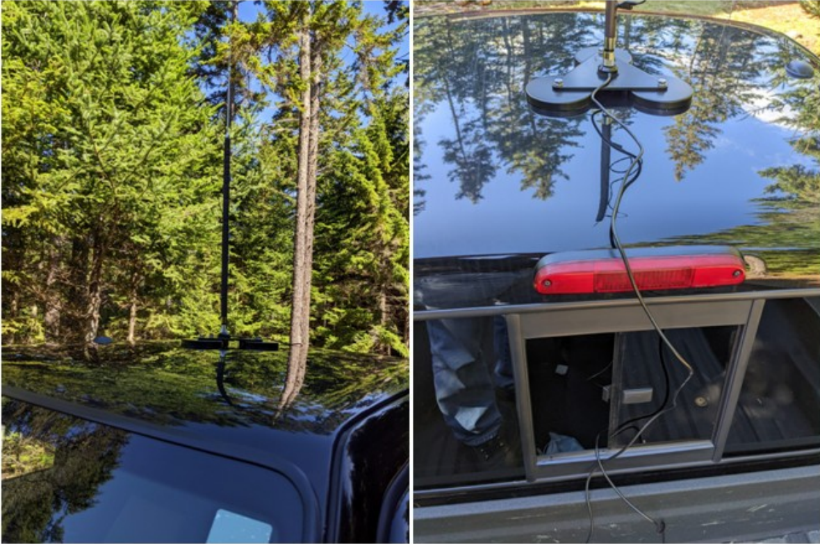
Antenna atop my truck and a close-up of the tri-mag mount.
