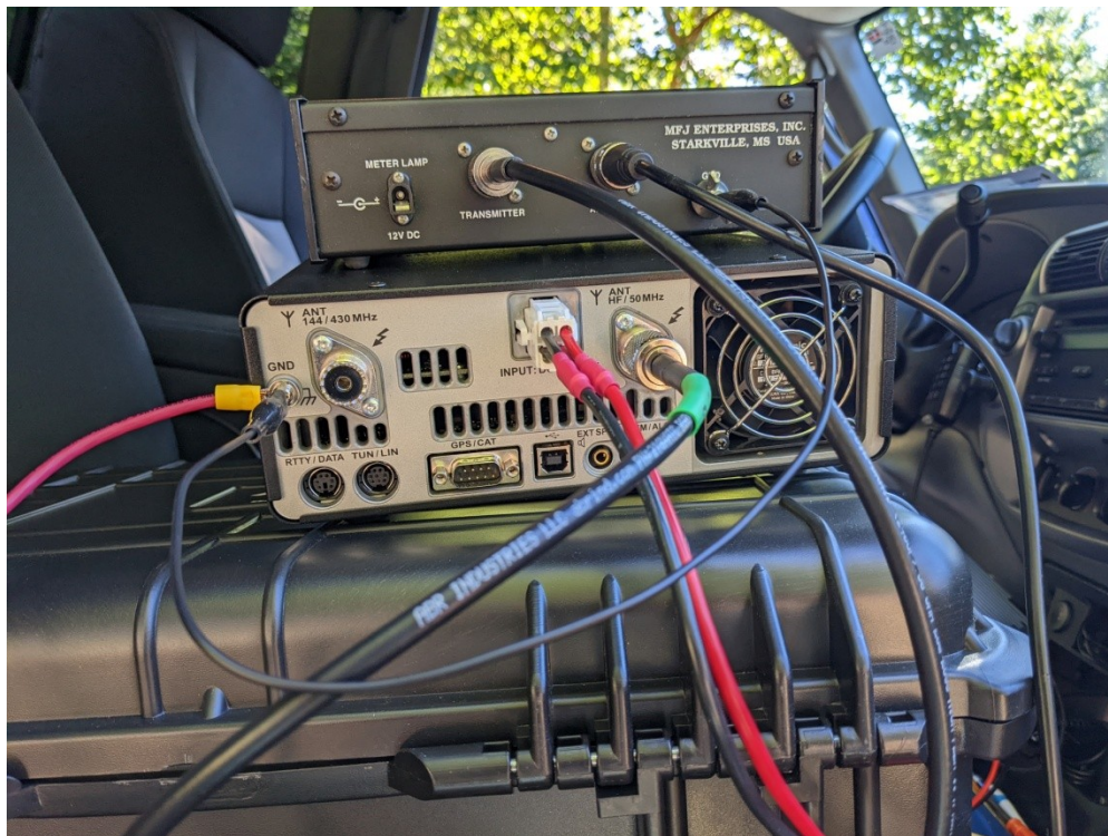
A view of the back of my radio and tuner set up for portable operations.
