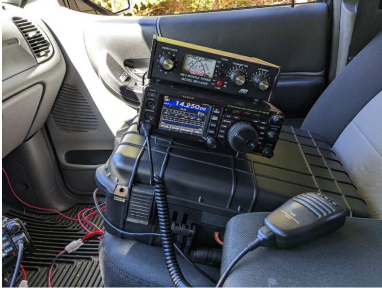
My radio and manual tuner set up on top of my go-box in my truck.
